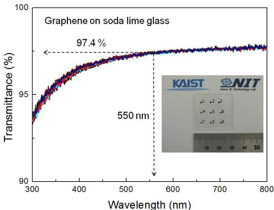
**Figure S2.** Optical transmittance curves at nine points of graphene on soda lime glass (as numbered in the inset). The inset shows the transferred graphene onto the soda lime glass (30 mm x 30 mm) as used to measure the optical transmittance. The optical transmittance is 97.4% at a wavelength of 550 nm, which coincides with the value for monolayer graphene.
