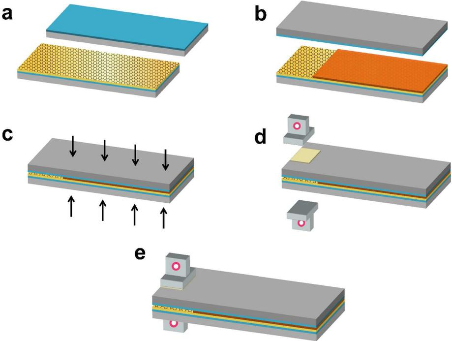
**Figure S3.** DCB specimen preparation procedures. (a) A silicon substrate containing graphene and a counterpart silicon substrate are cut with same size. (b) Applying epoxy adhesive on selected area of the substrate. (c) Attaching two substrates and curing under constant clamping pressure. (d) Aluminum loading tabs are attached with epoxy adhesive. (e) Completed DCB specimen.
