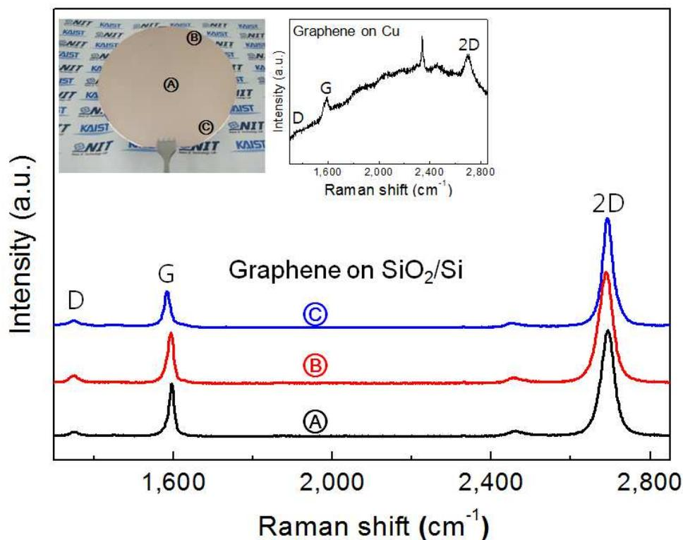
**Figure S1.** Raman spectra of three representative points (as denoted in the left inset) of graphene as transferred onto a SiO<sub>2</sub> (300 nm)/Si substrate. The left inset shows a photograph of the as-grown graphene on a 4-inch copper (300 nm)/SiO<sub>2</sub> (300 nm)/Si wafer. The Raman spectrum of the as-grown graphene on the copper surface is shown in the right inset.
