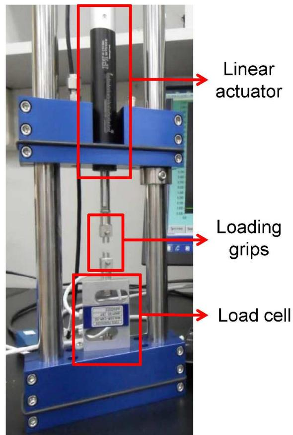
**Figure S4.** Photograph of the DCB test equipment.
